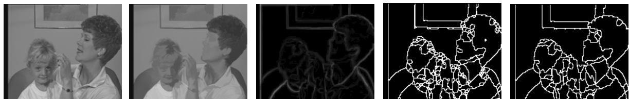
a) original image b) simplified image c) gradient image d) watershed image e) merged image
